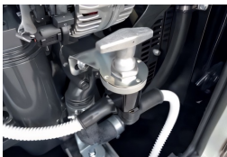
Batterieschalter Battery isolator switch
